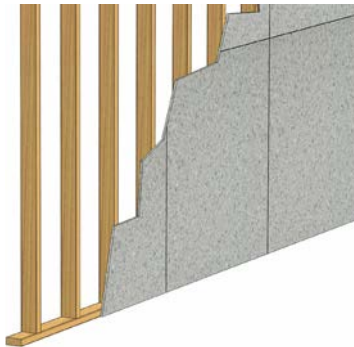
Wood studs faced with cement board
